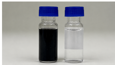
(b) From the left: Acetone phase after mild treatment, acetone phase after HDO.
