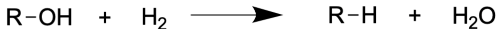
Figure 2.3: Hydrogenation reaction associated with catalytic hydrotreatment for bio-oil upgrading. Drawn on the basis of information from [2, 3].
