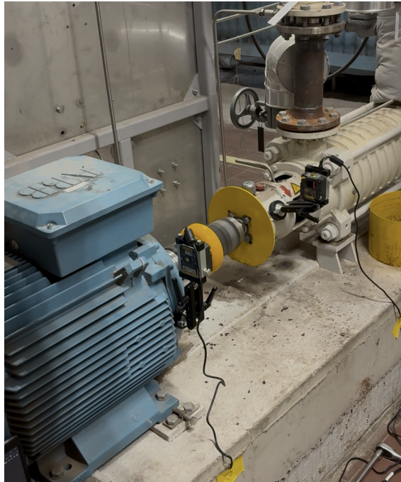
Figure 2.1: Easy Laser XT770 unit mounted on motor-pump setup.
