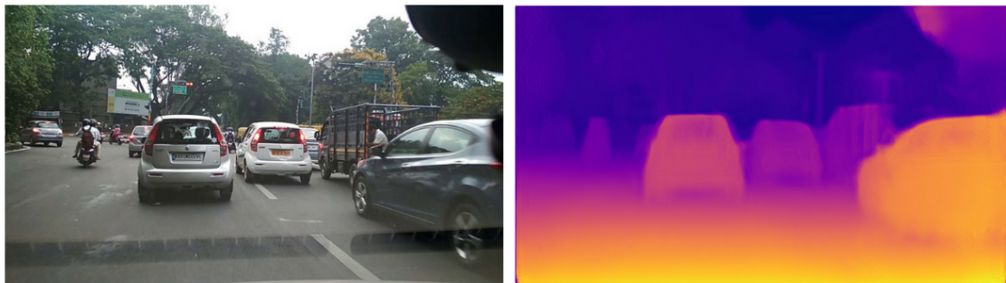
Figure 3.5: Depth map: the left is the original picture and the right is the correlating depth map. The farther the pixel is in 3D space, the darker the color is in-depth map
