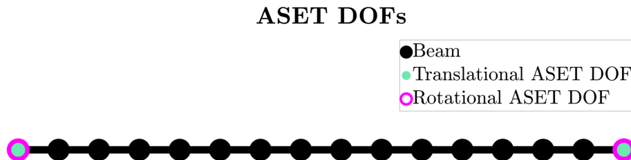
Figure 3.5: Illustration of ASET DOFs for the Guyan reduction example.
