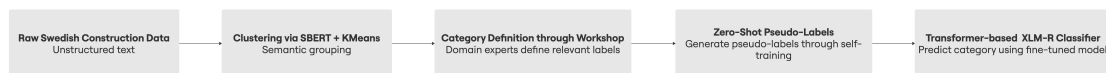
Figure 4.1: Overview of the 5 stages of implementation, including the 3 models, including, raw swedish construction data, clustering via SBERT + KMeans, category definition through workshop, zero-shot pseudo-labels and transformer-based XLM-R classifier.
