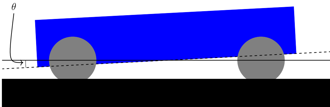
Figure 2.4: A pitch angle \theta around the car's lateral axis.
