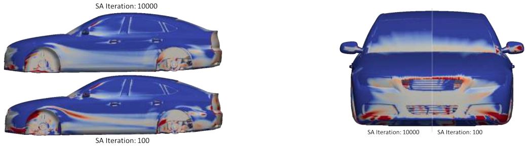
Figure 3.4: Comparison of sensitivity map for various SA iterations in DDES-based adjoint for fastback configuration
