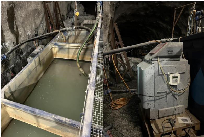
Figure 22 and 23. Collection container before discharge and automated ISCO sampler (Photo by the authors).
