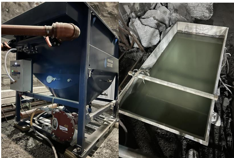
Figure 20 and 21. Lamella separator used for sedimentation and connected sludge container (Photo by the authors).
