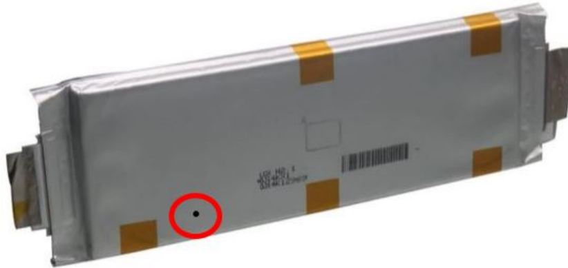
Figure 2.5: Illustration of puncture in pouch cell.
