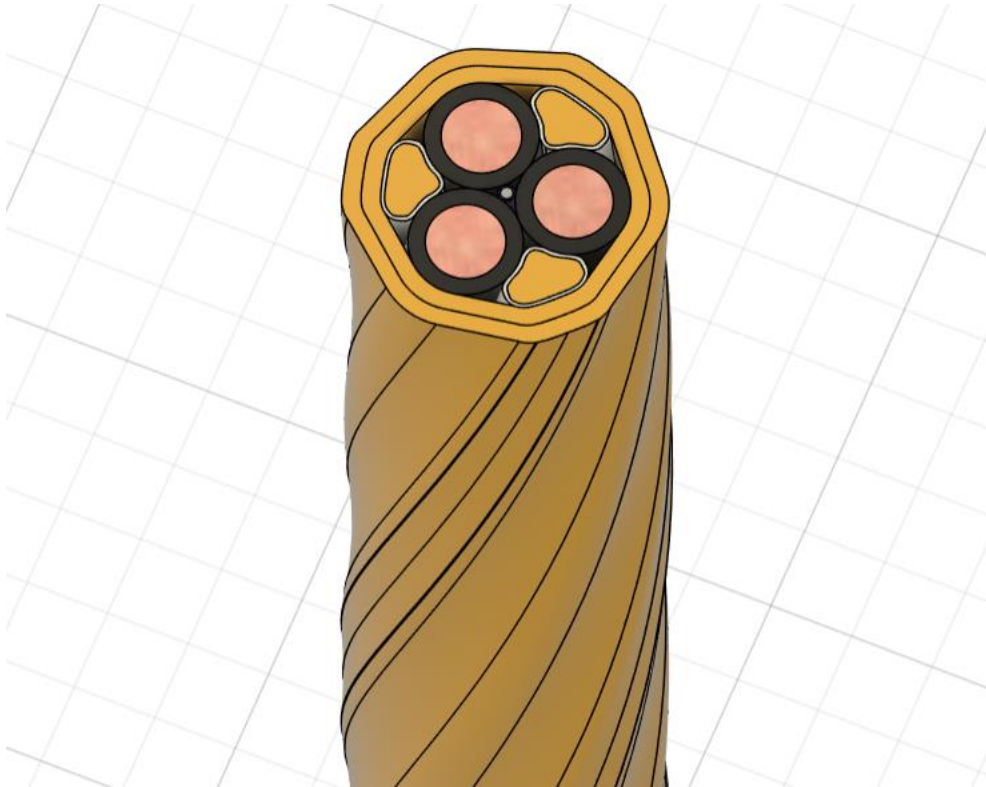
Figure 2: First draft extruded cable with desired twist in Fusion 360
