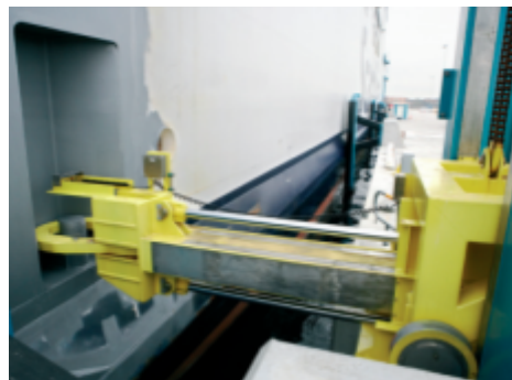
Figur 16. TTS Grip-based auto-mooring TTS Port Equipment AB (2012)
