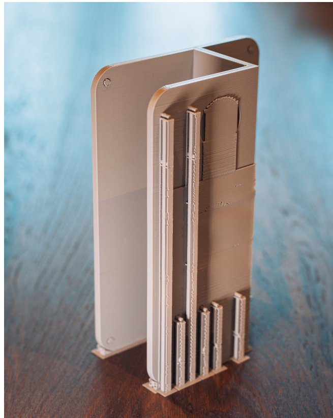
Figure 5.15: Bottom with supports
