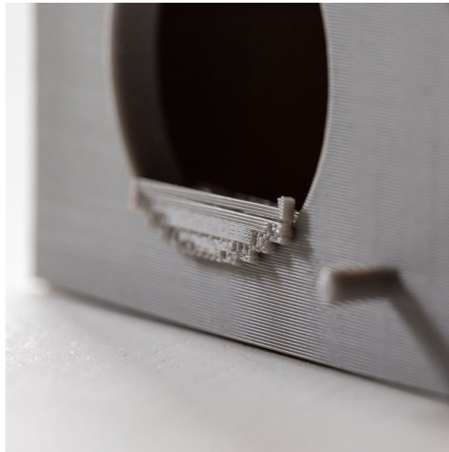
Figure 5.7: Support from 3D-printing
