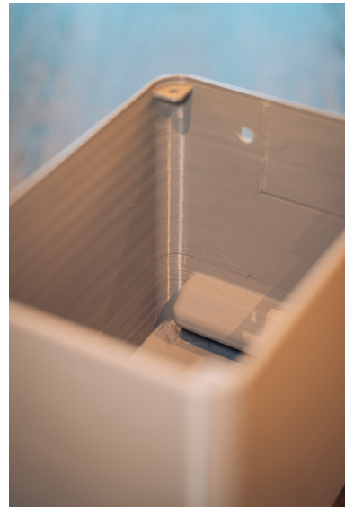
Figure 5.13: Inside the cover without supports
