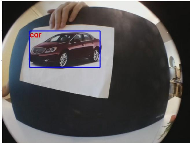
**Figure 4.2:** Example detection made by the computer vision module. A printed image of a car is held in front of the camera. It correctly identifies the image of a car.
