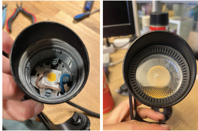
Figure 8.9: The LED ship and the lens
