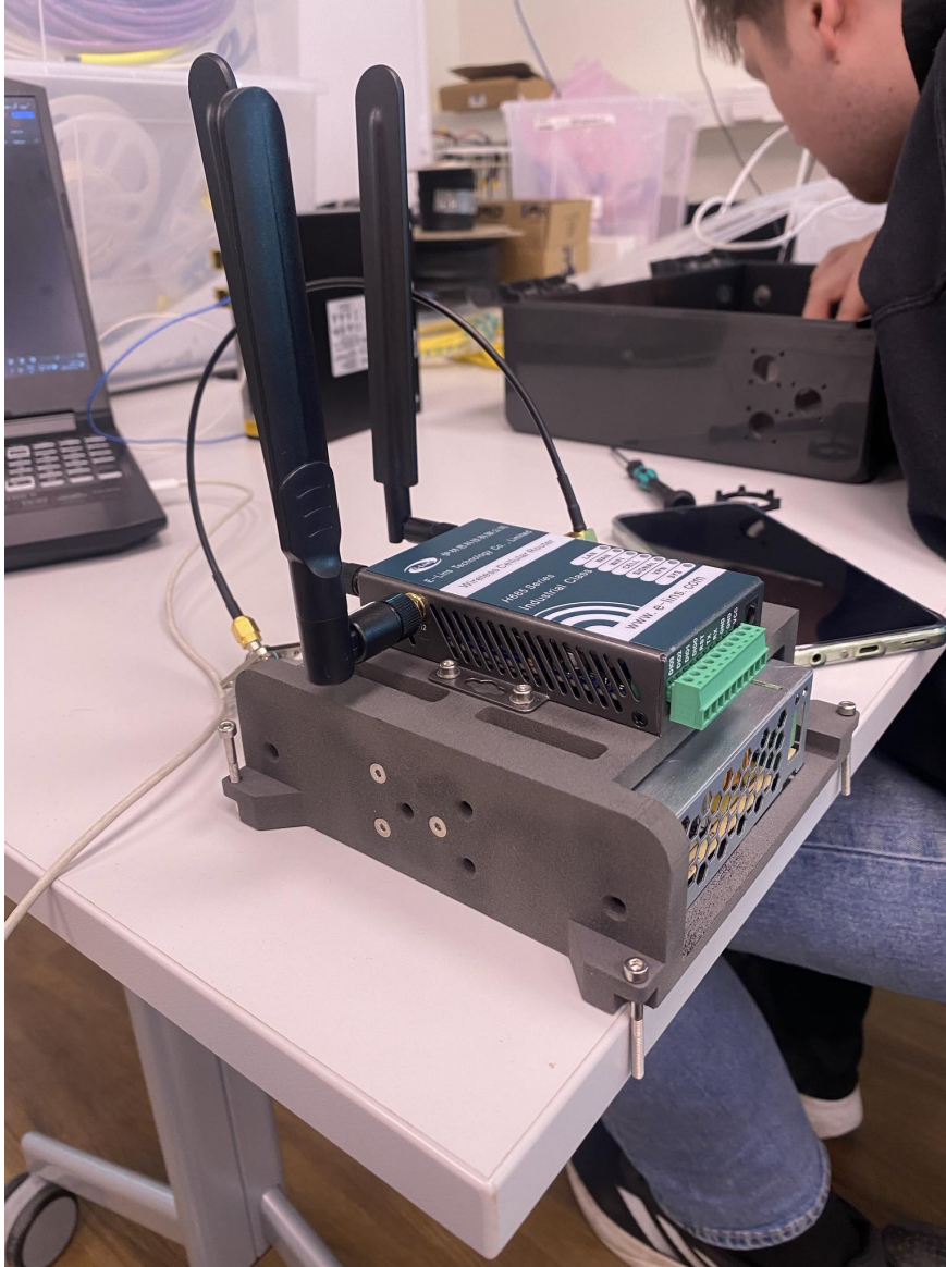
Figure B.2: The DC-DC charger and router bracket
