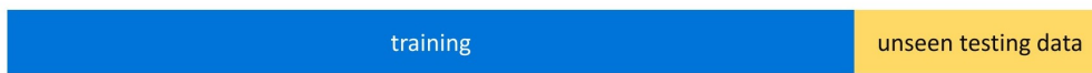
Figure 5.7: Evaluating the model on the data that was set aside before the construction of the model will give a result that reveals eventual overfitting, but is limiting due to the relatively small size of the testing set.
