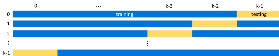
Figure 5.8: k -fold cross-validation will allow testing on, in total, a large number of data points, but it would be somewhat oblivious to overfitting. The order of the data points is randomized.
