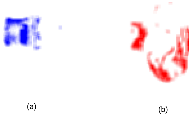
Figure 3.9: Coarse 2D Heatmap of part 3M2C (a) Sample 001 with Under-Extrusion (material removing) defect (b) Sample 014 with Over-Extrusion (material adding) defect
