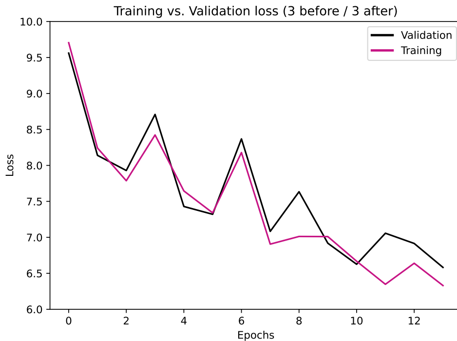
Figure 5.6: Training against validation loss for annotation configuration 4 (3 before / 3 after) trained for 14 epochs.
