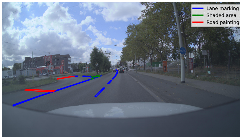
Figure 4.3: An image frame with lane marking (blue), shaded area (green) and road paintings (red) annotations.
