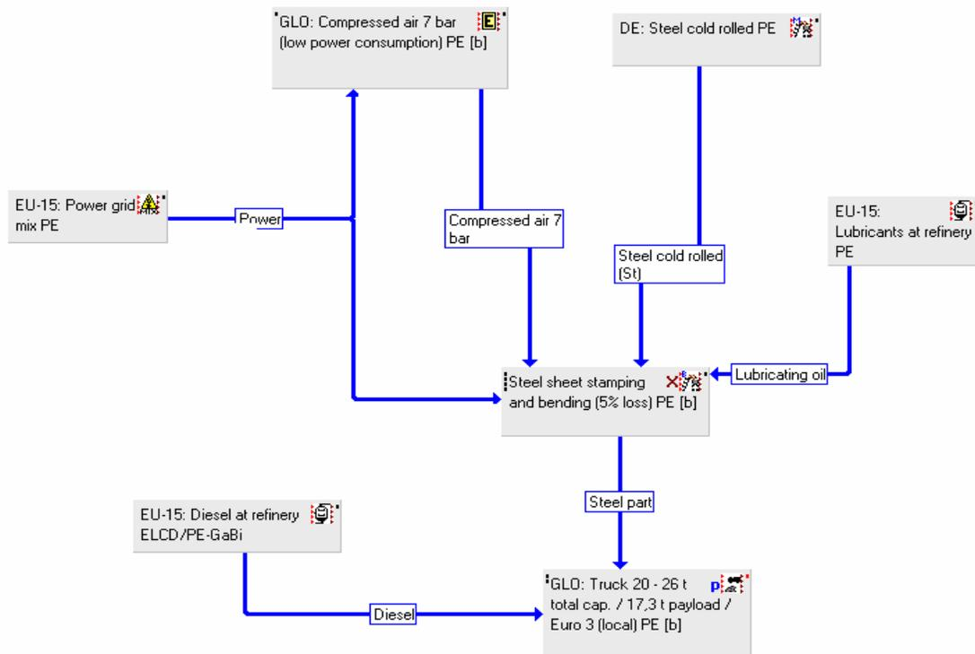
Figure 16 GaBi model for studs production
