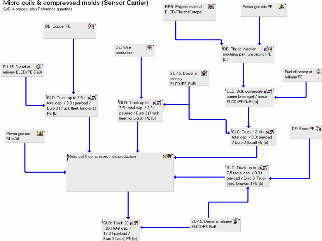
Figure 13 GaBi model for micro-coil (Sensor carrier) production
