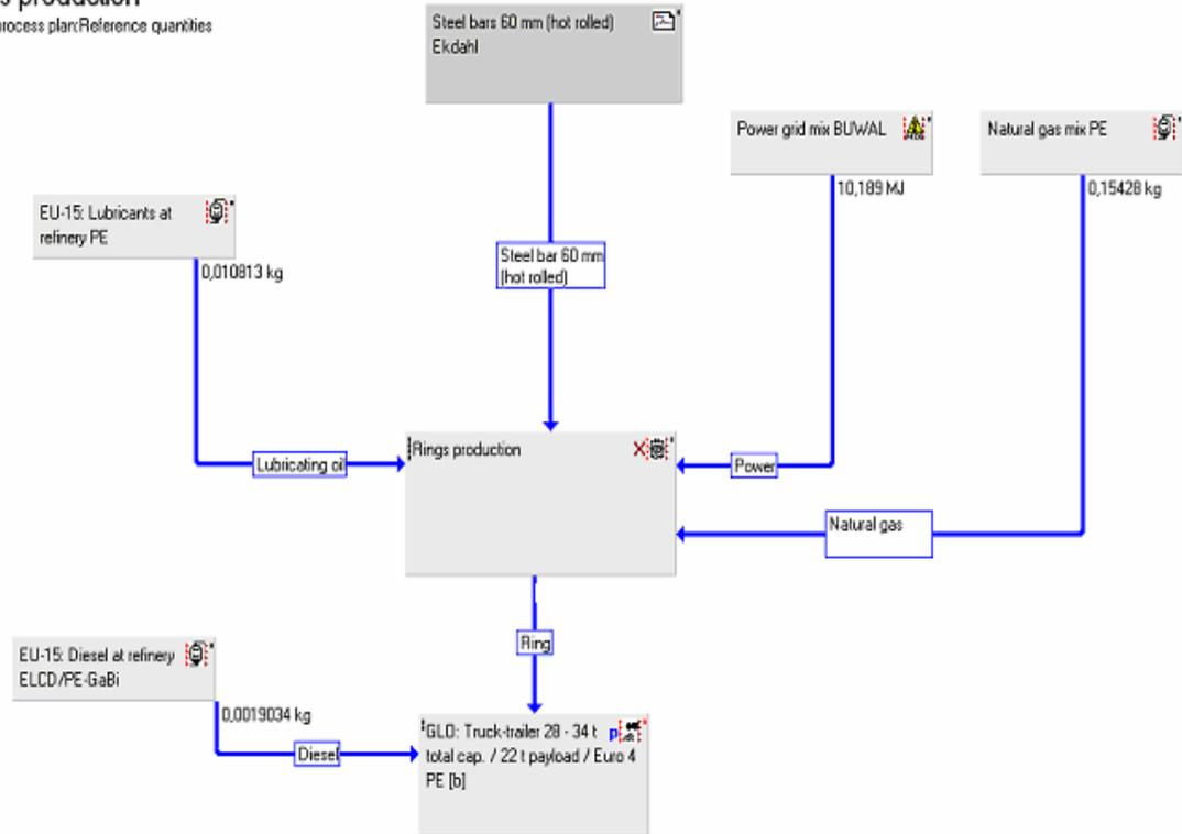
Figure 9 GaBi model for rings production
