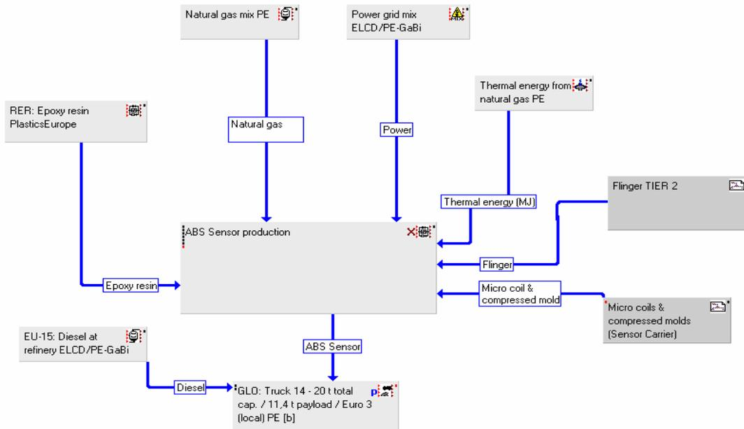
Figure 12 GaBi model for ABS Sensor production
