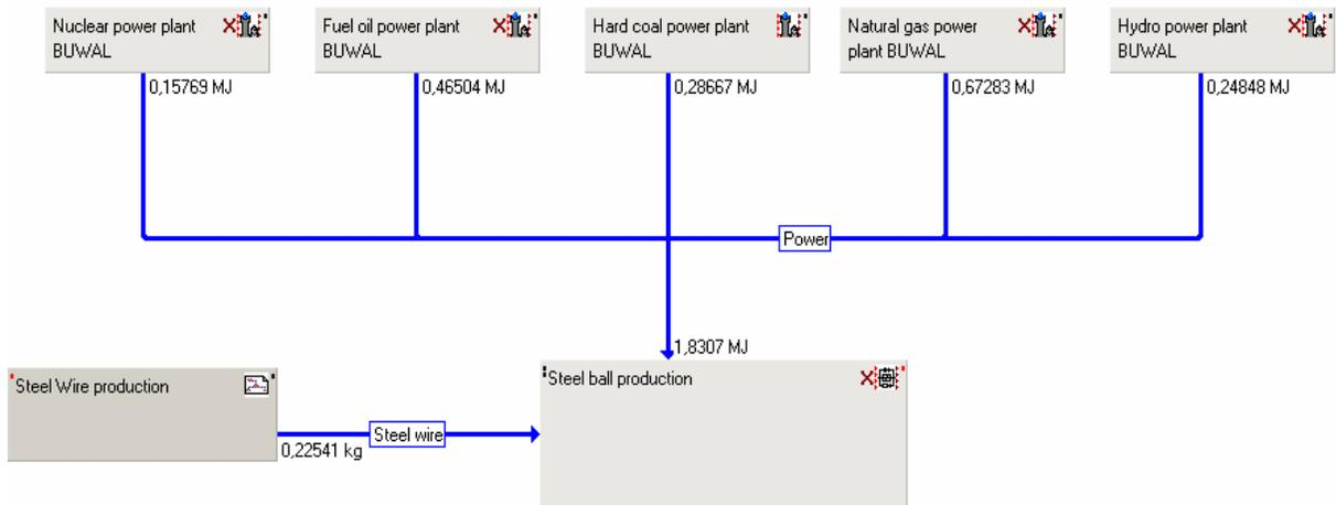
Figure 14 GaBi model for steel balls production
