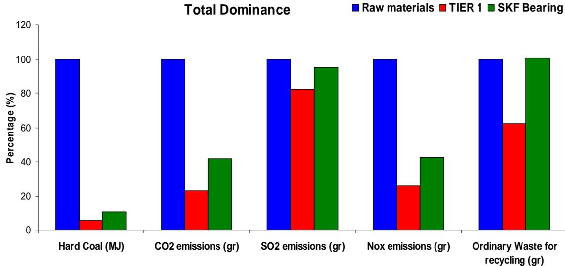
Figure 36 Total comparisons for the bearing's production system
