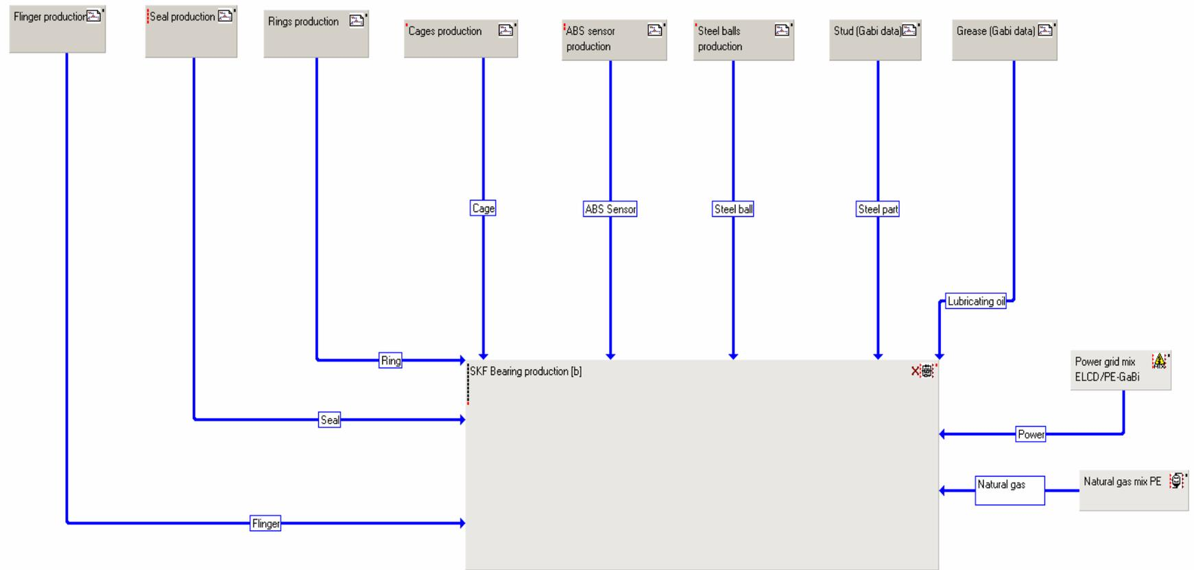
Figure 6 GaBi model for the production of the analysed bearing
