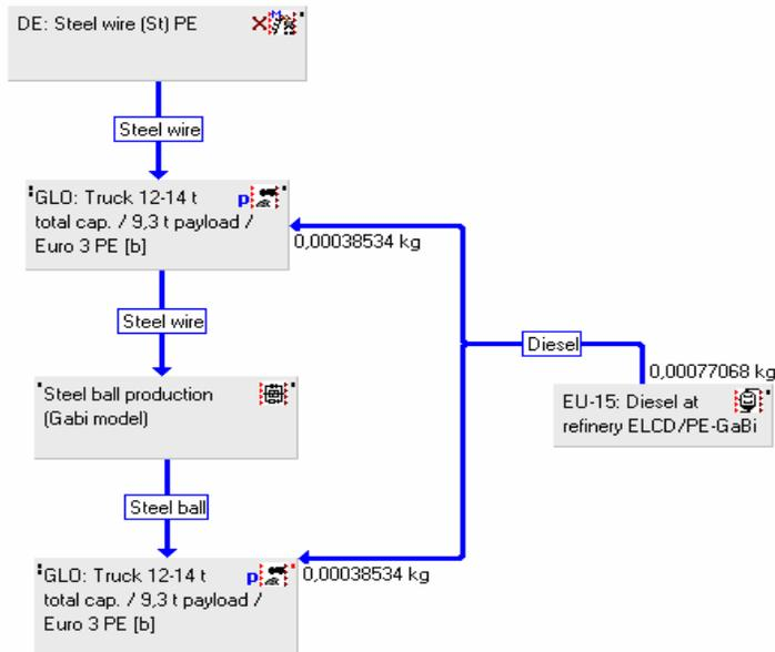
Figure 20 GaBi model for steel balls production
