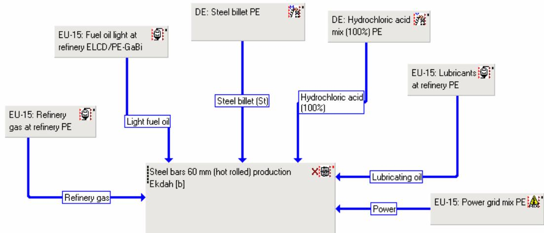
Figure 10 GaBi model for the steel bars production
