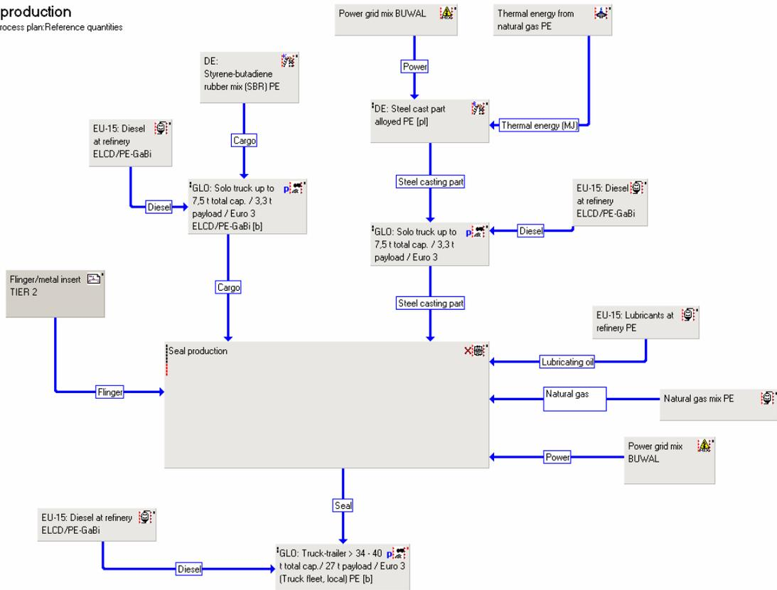
Figure 8 GaBi model for seal production
