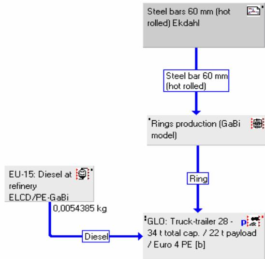
Figure 18 GaBi model for rings production
