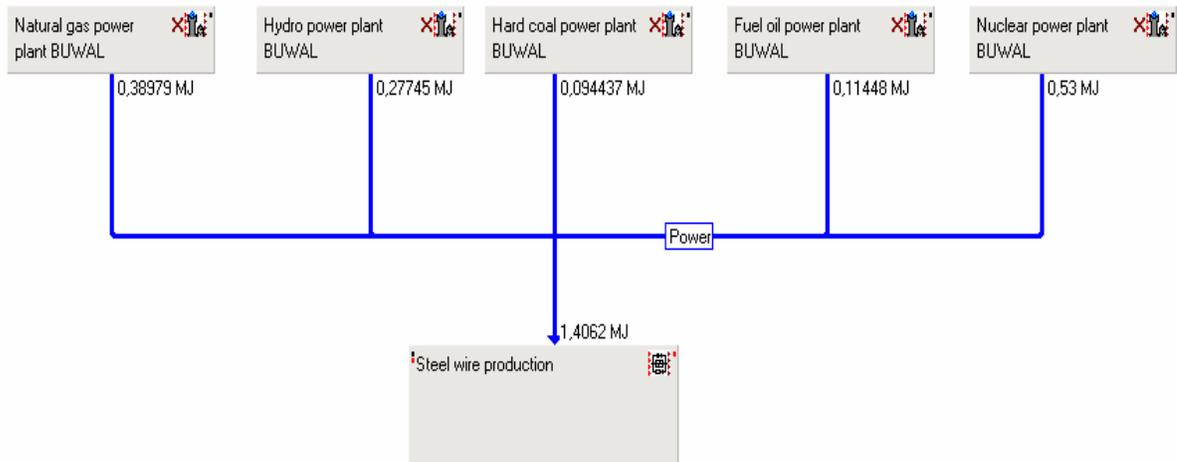
Figure 15 GaBi model for steel wire production
