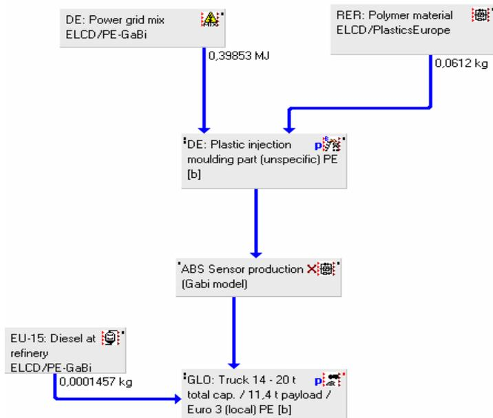
Figure 19 GaBi model for ABS Sensor production
