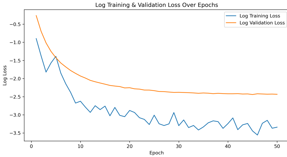
Figure A.2: Training and validation loss curves for FMROM implementation with principal component analysis and LSTM for surface elevation, U velocity and V velocity. The training halted after 50 epochs due to early stopping.
