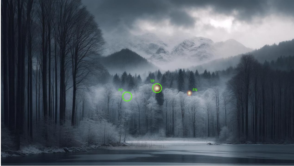
Figure 2.10: Examples of FP, FN, and TP predictions where the green circles are the predictions.
