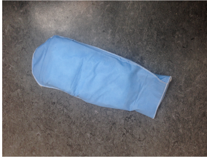
Figure 5.2: Thermal bag made of non-woven fabric and the material Thermal Wrap as an insulator.
