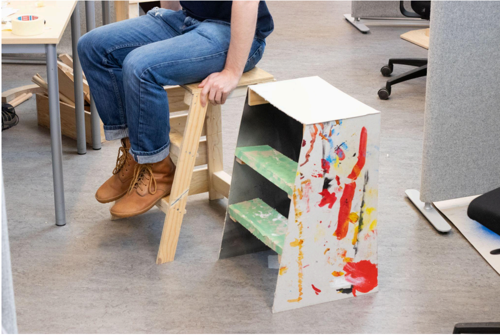
Figure 79. Mockups of the concept. First, a functional mockup in wood, followed by a cardboard mockup to examine how small it could be designed.
