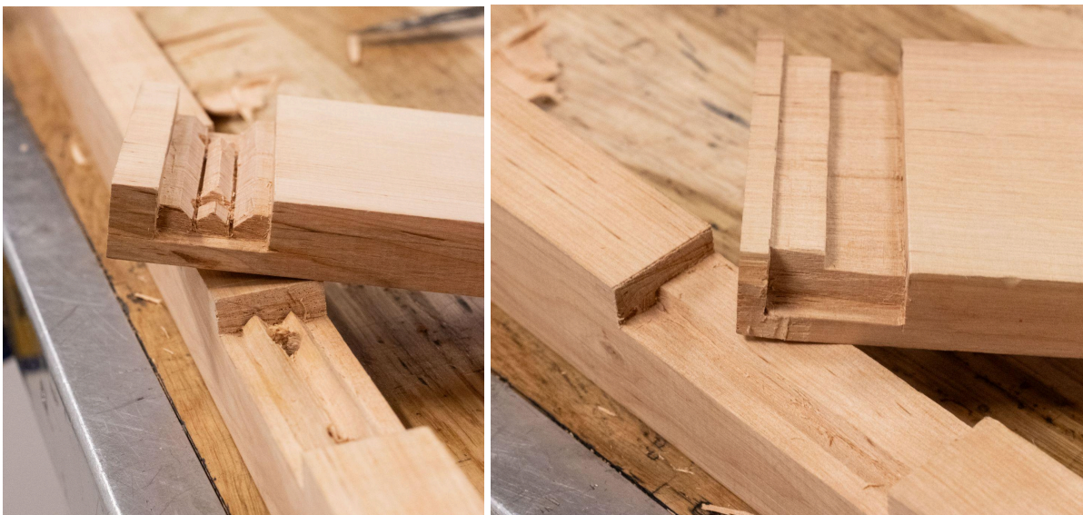
Figures 102 and 103. Prototypes of interior geometries to take the load of the screws.
