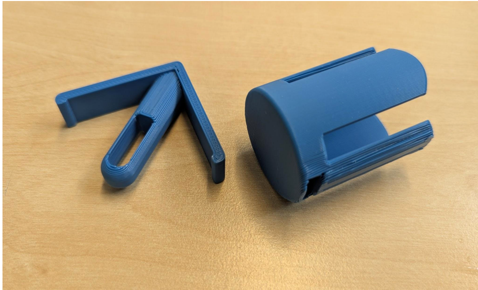
Figure 55. A corner connector where you can mount one or two sockets.
