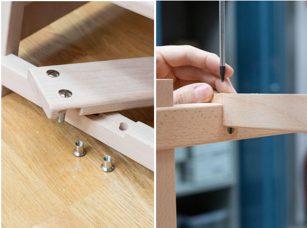
Figures 124 & 125. The two types of joints make Händig disassemblable and careable.
