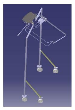
Figure 4.15: Concept 1: Isometric view
