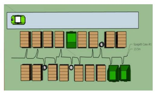
Figure 1.10: Spaghetti diagram of the operator path
