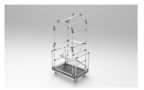
Figure 4.3: A solution developed to handle heavy hydraulic cables.
