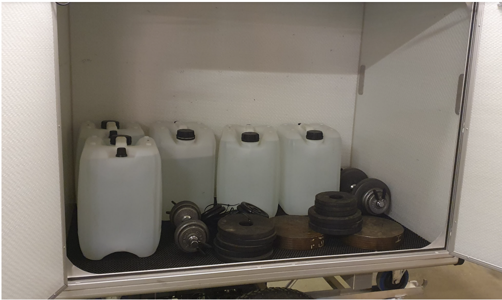
Figure 4.21: Bike container loaded with 200kgs
