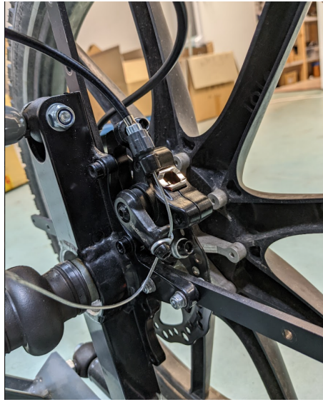
Figure 4.16: Brake calipers mounted on the bike
