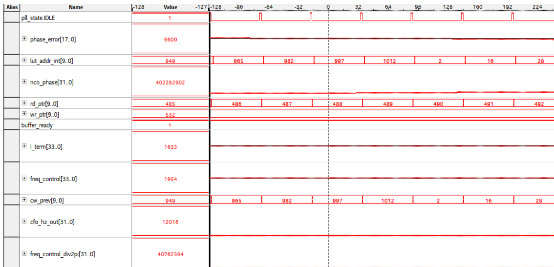
Figure 7.11: SignalTap waveform showing successful FPGA-based fixed-point DPLL operation and CFO lock at approximately 12 kHz.
