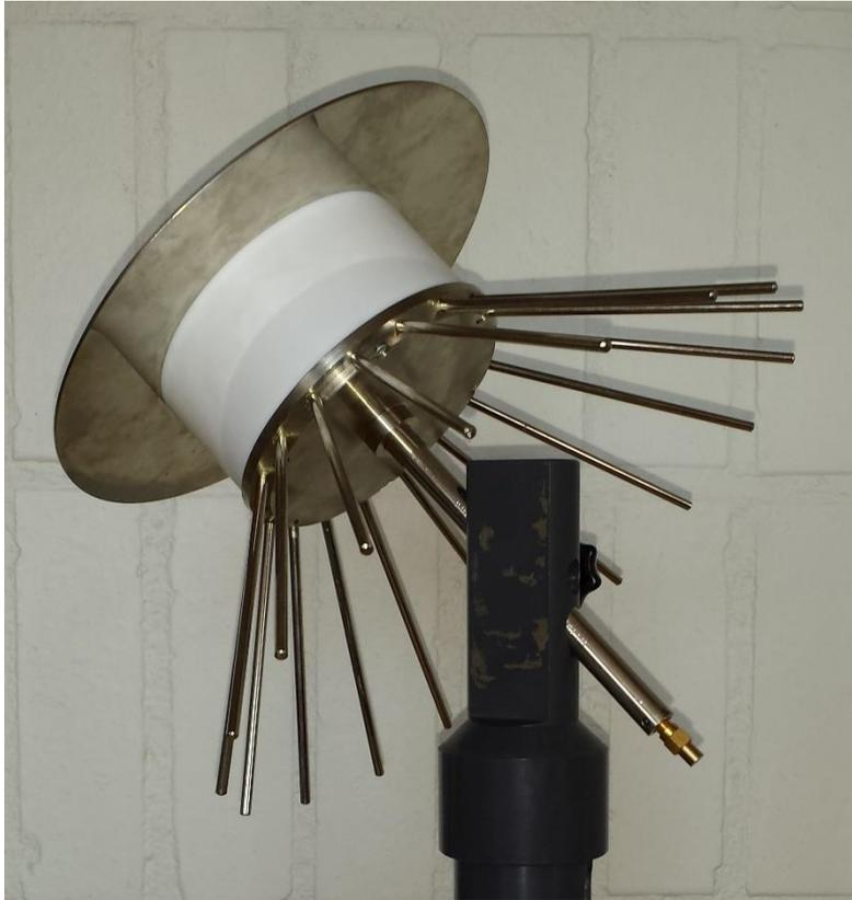
Fig. 18 Disc cone reference antenna used for calibrations
