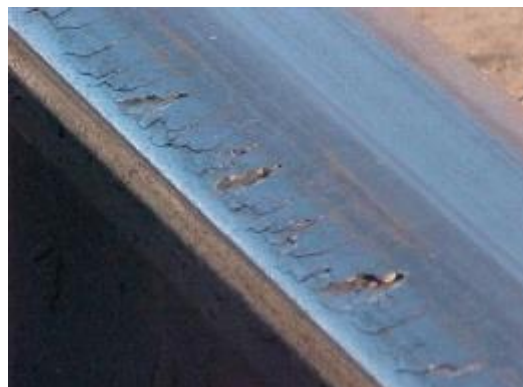
Figure 11: Gauge side head checking and flaking (from [12])
