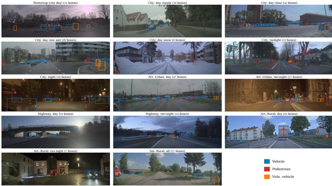
Figure 3.1: One representative frame per stream segment of the city-day-curated manifest, with target-class bounding boxes overlaid (Vehicle in blue, Pedestrian in red, VulnerableVehicle in orange; per-panel legend shown in the lower right). The top-left panel shows the bootstrap prefix; the remaining thirteen panels follow the stream order of Table 3.2 (left-to-right, top-to-bottom), with the panel title naming the block and the number of bounding boxes drawn. Within the early city-day rows, transitions hold structural metadata ( road_type , time_of_day ) constant while the weather bucket changes. Across the later rows, road type and time of day also shift, producing the intended sequence of domain changes.
