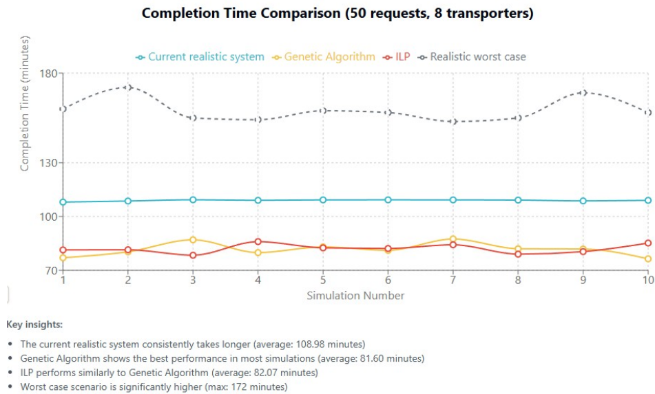
Figure 5.6: Completion time for each simulation with eight porters and 50 requests, the realistic algorithm line is the median of 1000 runs, the worst case is the worst run of the 1000 realistic runs.
