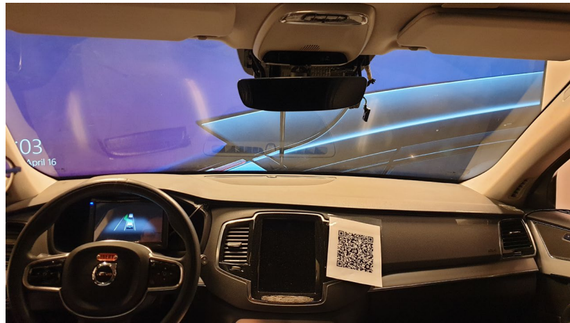
Figure 23. View from inside the simulator showing the outside TV screens and the DIM display.
