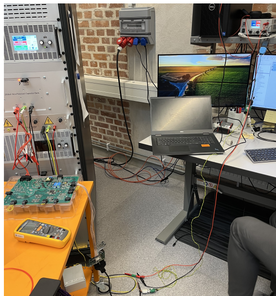
Figure 3.4: The setup in the lab with the lab-rack-insulation-module to the left, the power source for the boards up to the right and the computer for measuring/-analyzing.
