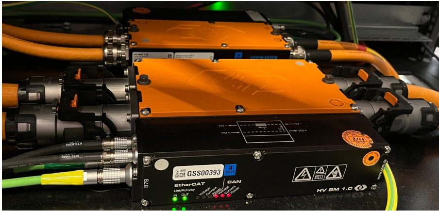
Figure 3.6: HV Breakout Modules 1.2 to handle pole-to-pole voltage.
