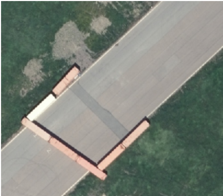
Figure 3.13: Real-world test site, containers are placed on an airport landing strip. Not shown in the picture are road barriers, approximately 1 meter tall, extending the containers at the time when the data was recorded.
