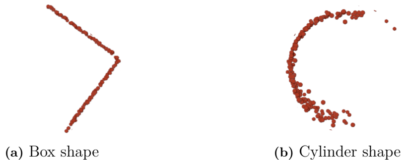
Figure 5.2: Top-view of an aggregated point cloud for a box corner and a cylinder. The reconstruction of the cylinder shape is pretty good, but not as good as the box corner.
