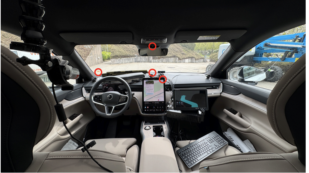
Figure 4.4: Overview of the four calibration points.
