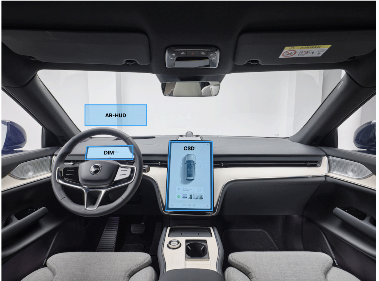
Figure 3.1: Placement of AR-HUD, DIM and CSD.
