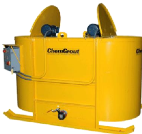
Figure 3.3 Agitator in tunnel injection grouting.
