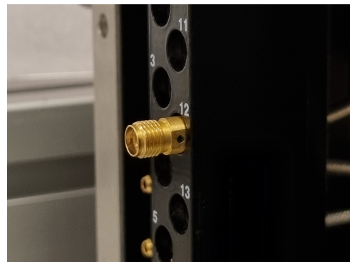
Figure 3.11. Type of socket used for Test 4. Outer diameter of threads \approx 6.25 mm.
