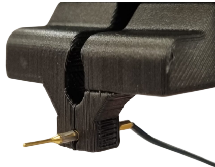
Figure 5.7. Gripper holding the cable in Test 2.
