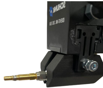
Figure 5.5. Gripper holding coaxial RF cable.
