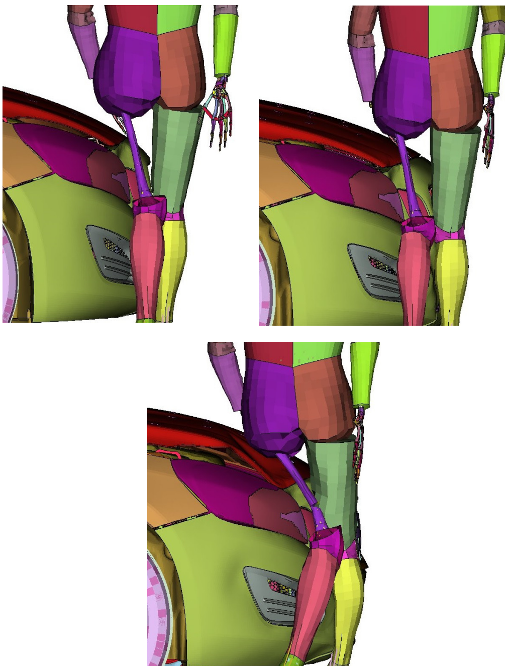
Figure 4.19: Fracture of femur at maximum tibia bending moment at 25km/h (top left), 40km/h (top right) and 50km/h (bottom) for impact point P5
