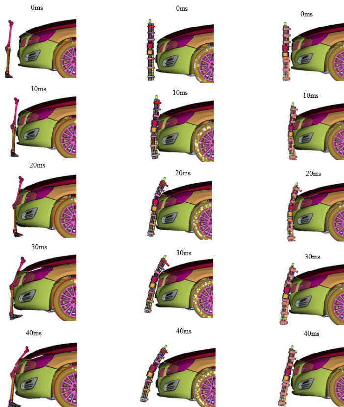
Figure 4.1: Kinematic behaviour of THUMS impact leg and Flex-PLI collision with vehicle, THUMS impact side leg (left), Flex-PLI (75mm above ground, middle), Flex-PLI (walking position, right)
