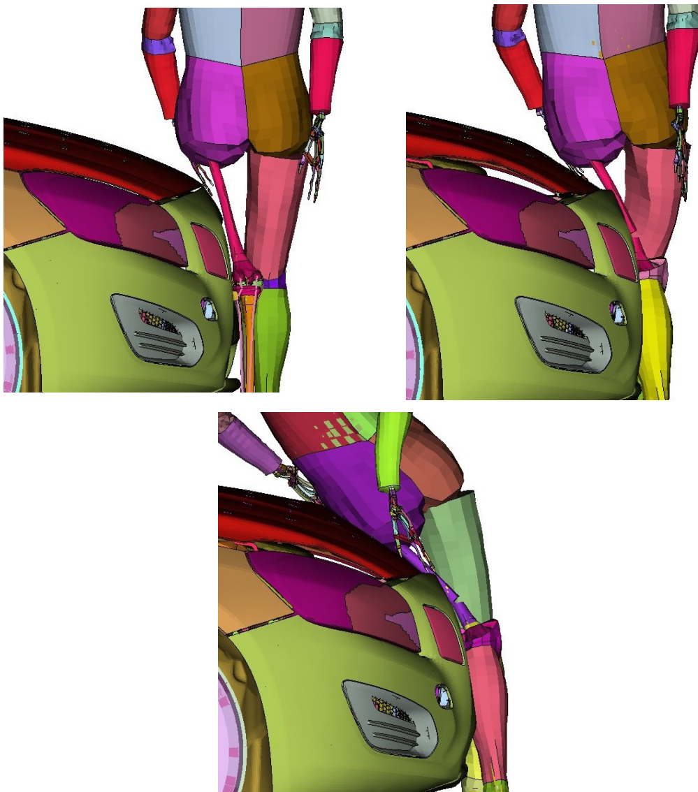
Figure 4.18: Fracture of femur at maximum tibia bending moment at 25km/h (top left), 40km/h (top right) and 50km/h (bottom) for impact point P3
