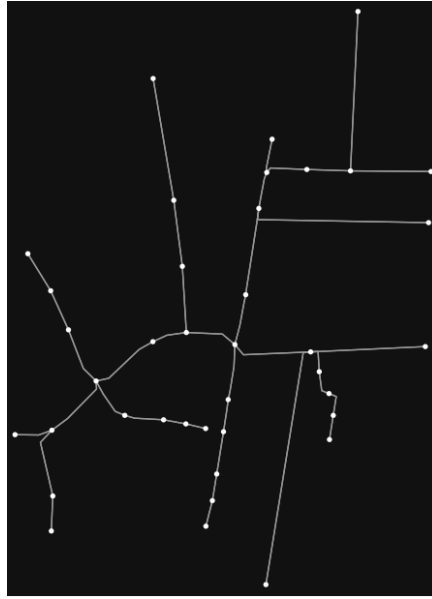
Figure 5. Example of a map gathered from OpenStreetMap and then simplified to represent an SD map. The dots are nodes, and the lines connecting them are edges.
