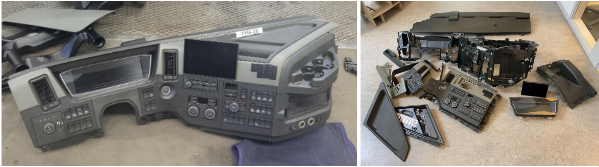
Figure 13. FM Electric instrument panel. Figure 14. Partially dismantled instrument panel.
