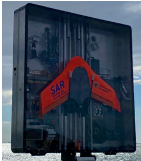
Figure 1.1: The fixed-wing drone used by the SSRS in a combined launcher, display and recharge device. This image was provided by the SSRS
