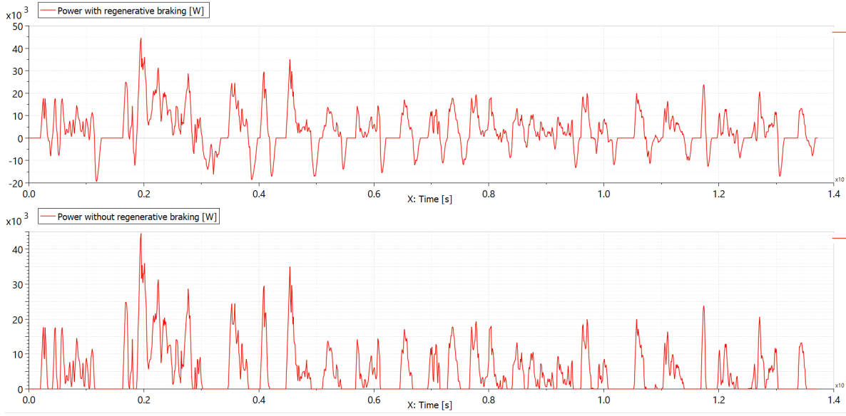
Figure 10: Regenerative braking in UDDS driving cycle compared to mechanical braking
