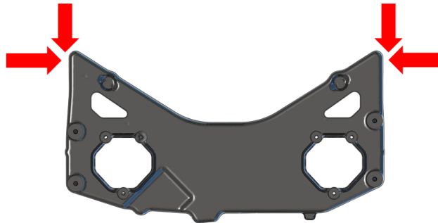
Figure 3.2: Illustration of crash scenario 1. Note that the loads on the left and right side are applied in two separate load cases.
