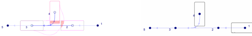
Figure 2.2: Traffic rule illustration: On the left, a potential collision may occur between two vehicles. On the right, after implementing a traffic rule that blocks segment (2,3) when a vehicle is positioned at point 4, the collision is effectively prevented because the other vehicle is prohibited from entering segment (2,3).
