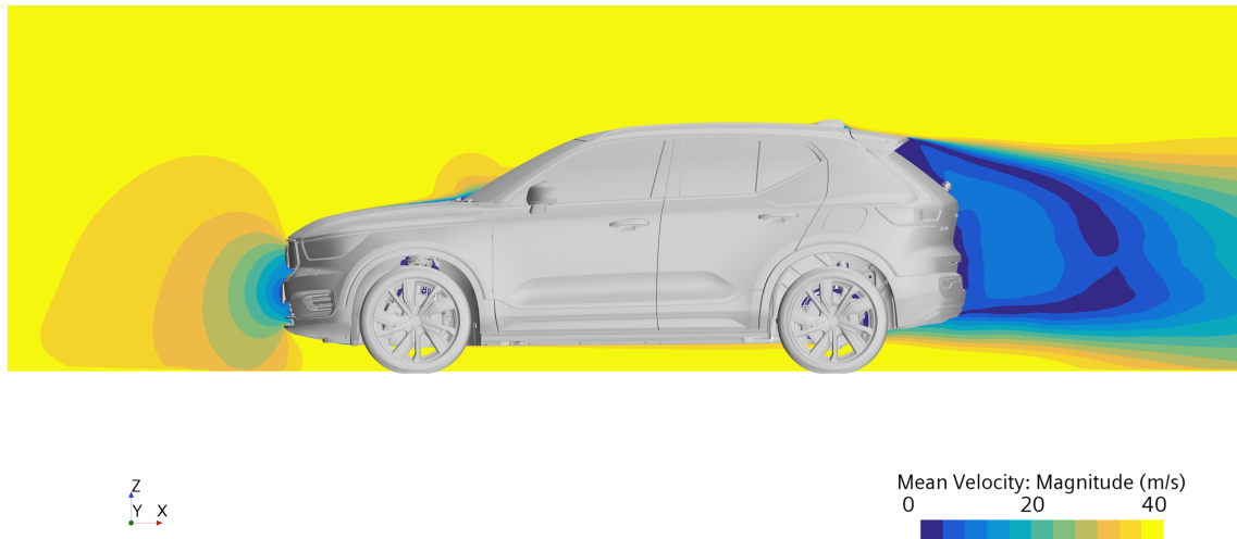
Figure 4.14: Scalar scene of the high turbulence simulation showing the mean velocity magnitude of the XC40, side-view
