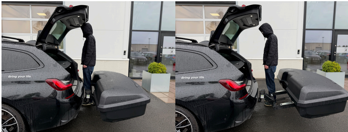
Figure 34: Illustration of the increased space between the car and the box facilitated by the new slide function, with a person standing in between as reference. (Author's own image)
