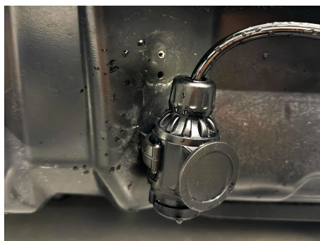
Figure 31: A tool clamp has replaced the cable holder. (Author's own image)
