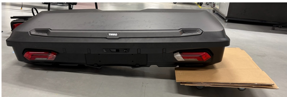
Figure 20: A low-profile trolley was placed under one side of the box simulating a canoe cart. (Author's own image)
