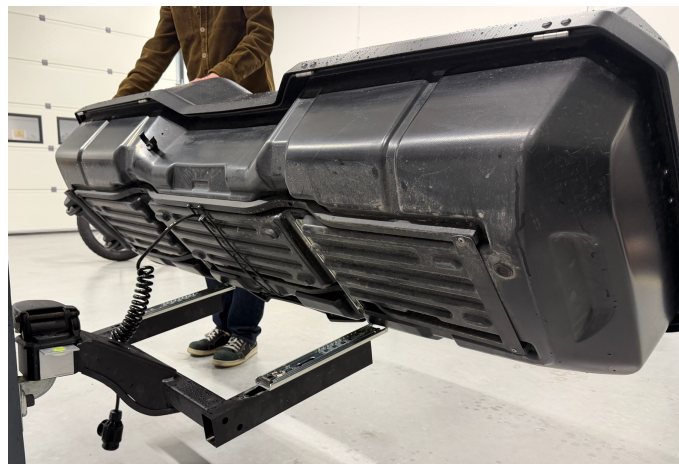
Figure 23: The tilt function was evaluated by simply tilting the box on the platform. (Author's own image)
