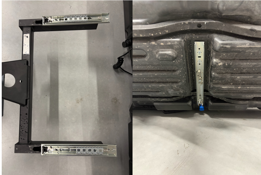
Figure 24: One part of the slide was mounted to the platform and the other to the underside of the box. (Author's own image)
