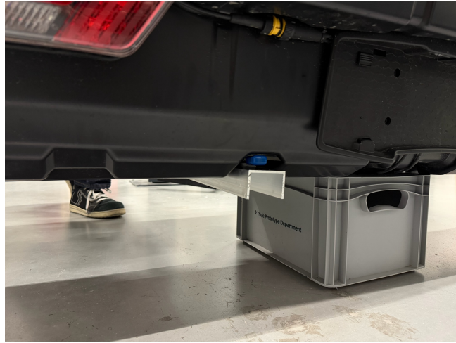
Figure 17: U-profiles were test-mounted on the underside of the box. (Author's own image)
