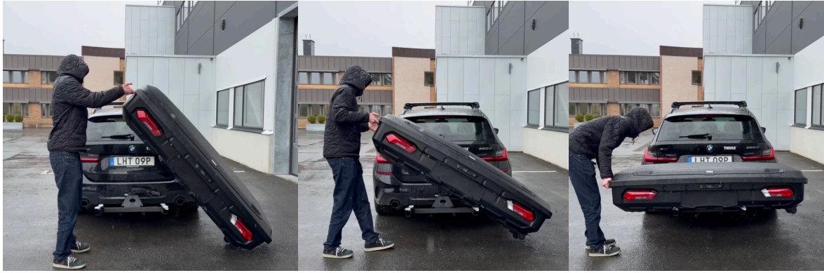
Figure 36: Series of pictures illustrating how the wheels allow the user to lay the box on the platform instead of lifting it. (Author's own image)
