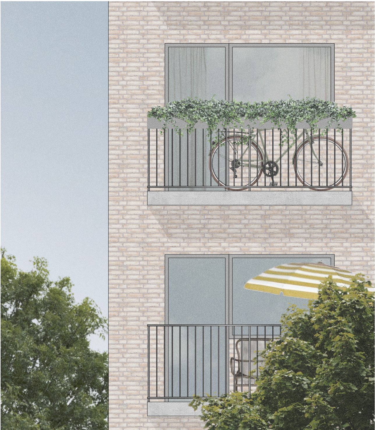
Illustration of facade with cantilever balconies.
