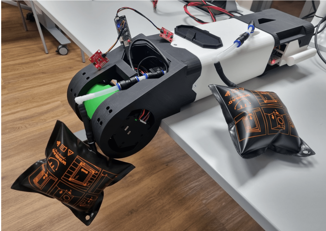
Figure 4.2: As-built RPK prototype at the time of writing, documenting the physical integration state used during iterative testing. The image shows temporary pump wedges used during prototyping in place of the final air-chamber sleeves; the complete shin-side 3D-printed components are not shown in this view.
