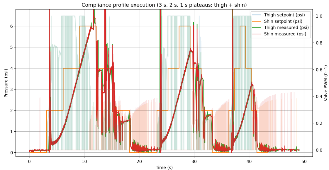
Figure 5.9: Compliance profile execution for thigh and shin commanded simultaneously: 0 \rightarrow 2 \rightarrow 4 \rightarrow 6 \rightarrow 4 \rightarrow 2 \rightarrow 0 psi, performed for three cycles using 3 s, 2 s, and 1 s plateaus per level. Faint lines on the secondary axis show valve PWM activity.
