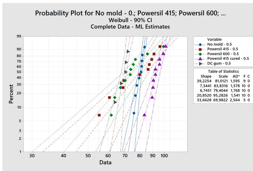
**Figure 4.5:** Weibull distribution of breakdowns in 0.5 mm polyethylene film with different mold around the spherical electrodes
