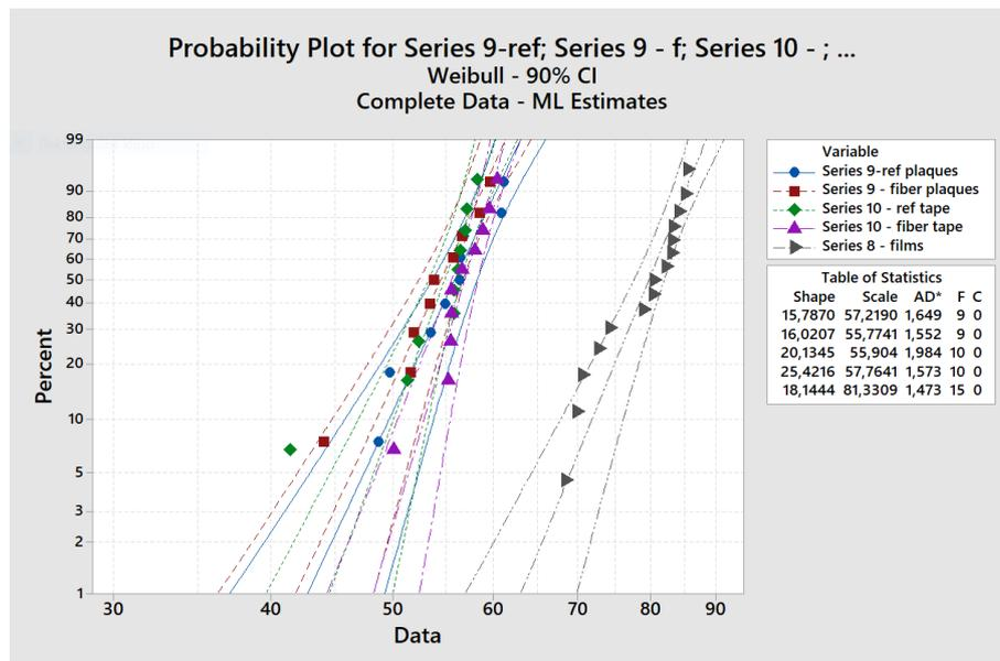
**Figure 4.12:** Weibull distribution of breakdowns in plaques and tape vs breakdowns in polyethylene films.
