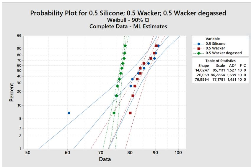
**Figure 4.2:** Weibull distribution of breakdowns in 0.5 mm polyethylene films in silicone and Wacker oil with standard electrodes.
