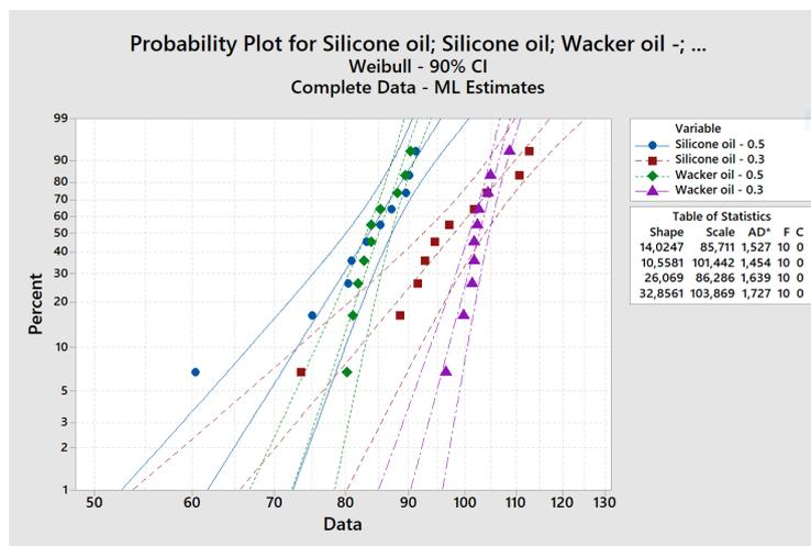
**Figure 4.7:** Weibull distribution of breakdowns in 0.5 mm and 0.3 mm polyethylene films with standard electrodes in both Silicone oil and Wacker oil.
