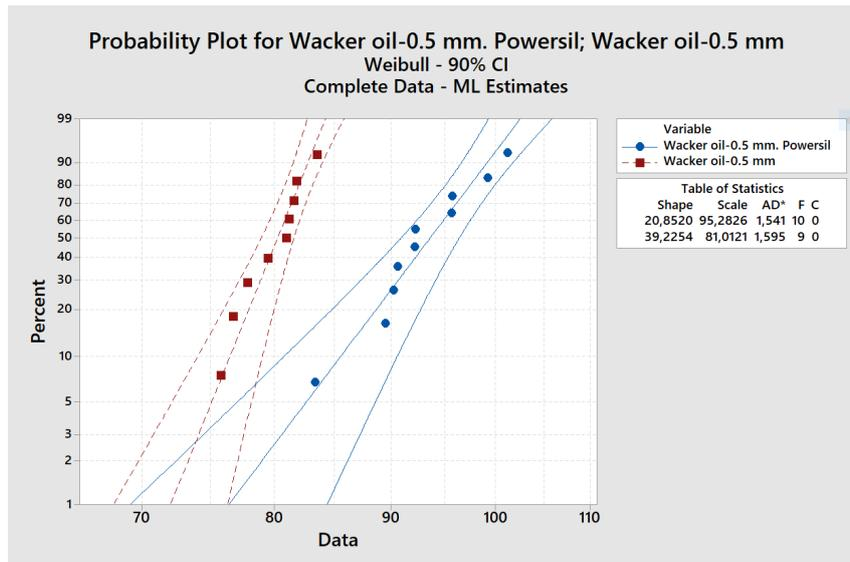
**Figure 4.4:** Weibull distribution of breakdowns in 0.5 mm polyethylene films in Wacker oil with Powersil 415 cured electrodes and spherical electrodes without mold.
