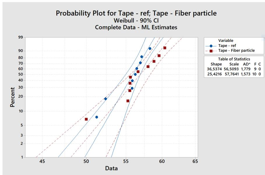
**Figure 4.11:** Weibull distribution of breakdowns in tape with and without fiber particles in it
