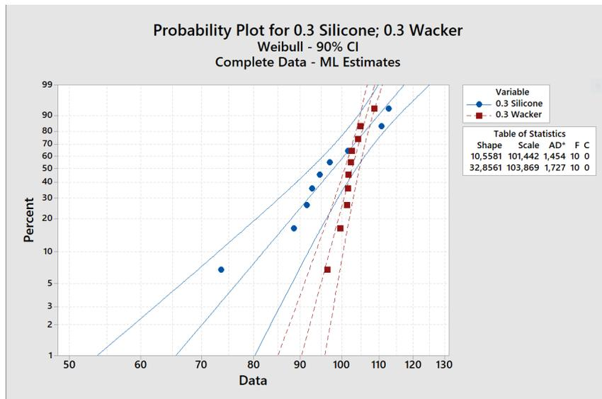
**Figure 4.1:** Weibull distribution of breakdowns in 0.3 mm polyethylene films in silicone and Wacker oil with standard electrodes.
