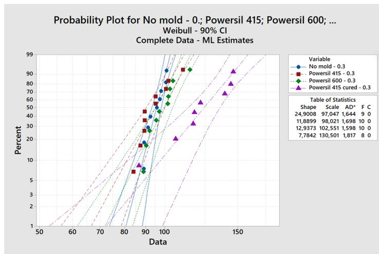
**Figure 4.6:** Weibull distribution of breakdowns in 0.3 mm polyethylene film with different mold of silicone gum around the electrodes.
