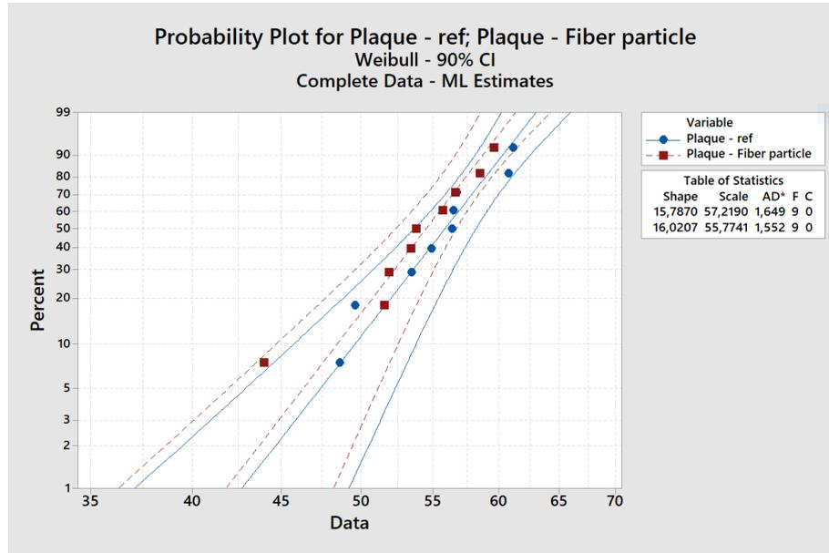
**Figure 4.10:** Weibull distribution of breakdowns in plaques with and without fiber particles in it.
