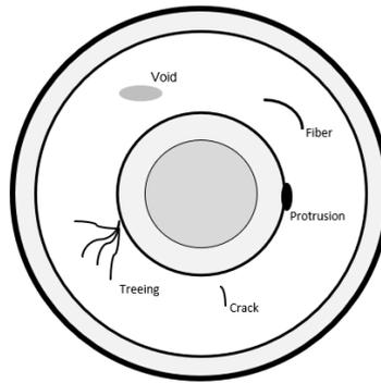
**Figure 2.2:** Schematic view of defects that may occur in a cable.
