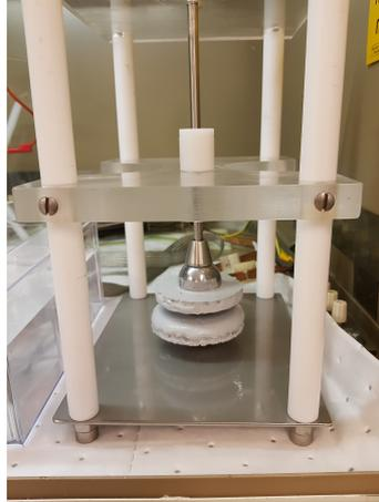
**Figure 3.5:** Spherical electrodes moulded in Powersil 600 A-B for series 5.
