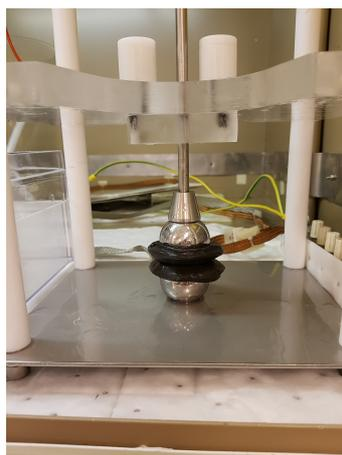
**Figure 3.4:** High voltage test rig with spherical electrodes moulded in uncured Powersil 415 for series 4.
