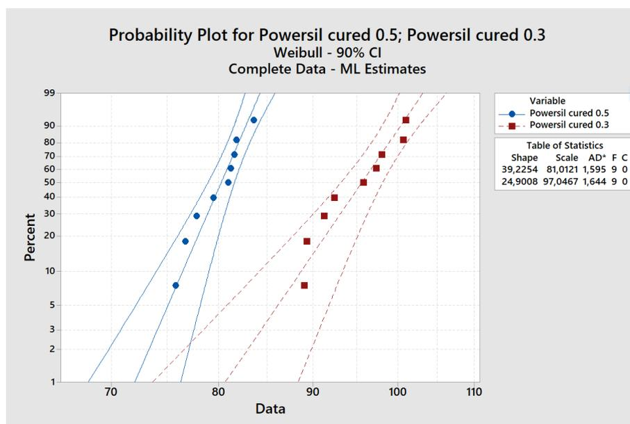
**Figure 4.9:** Weibull distribution of breakdowns in 0.5 mm and 0.3 mm polyethylene films with cured Powersil 415 electrodes and Wacker oil
