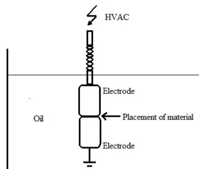
**Figure 2.3:** Schematic view of an example test rig for high voltage testing.
