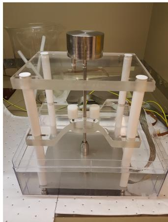
**Figure 3.1:** High voltage test rig with standard electrodes.
