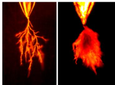
**Figure 2.1:** Electrical treeing from a sharp edge.
