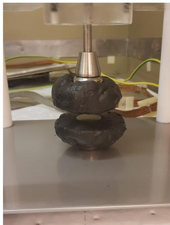
**Figure 3.6:** Spherical electrodes moulded in cured Powersil 415 for series 6.
