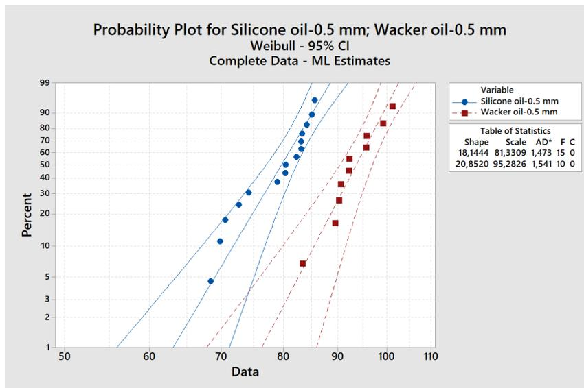
**Figure 4.3:** Weibull distribution of breakdowns in 0.5 mm polyethylene films in silicone and Wacker oil with Powersil 415 cured electrodes.
