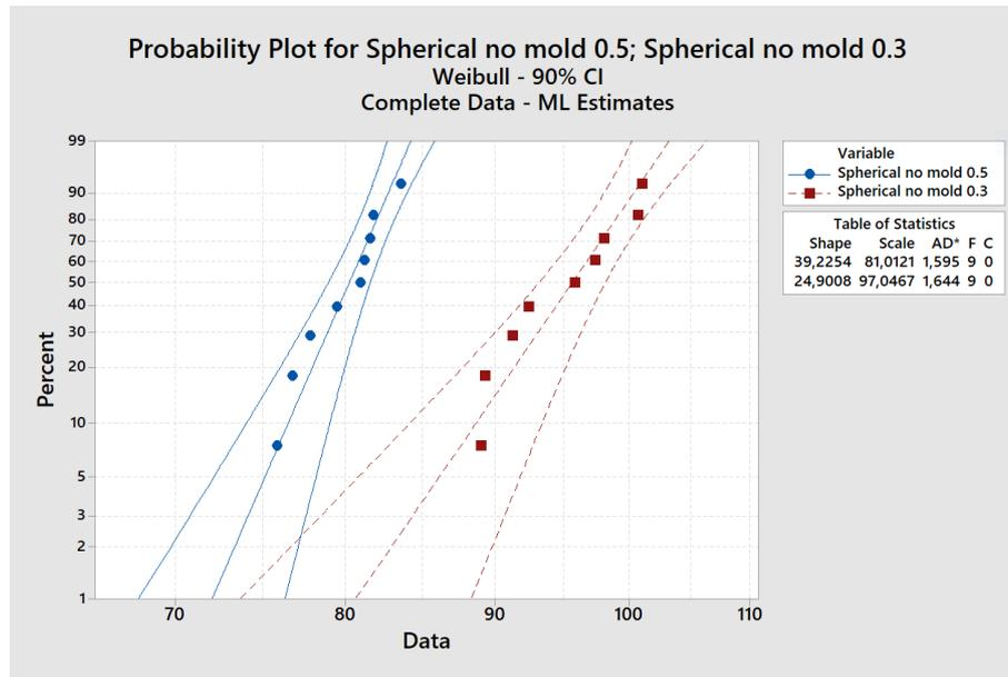
**Figure 4.8:** Weibull distribution of breakdowns in 0.5 mm and 0.3 mm polyethylene films with spherical electrodes and Wacker oil.
