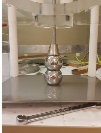
**Figure 3.3:** High voltage test rig with spherical electrodes for series 3.
