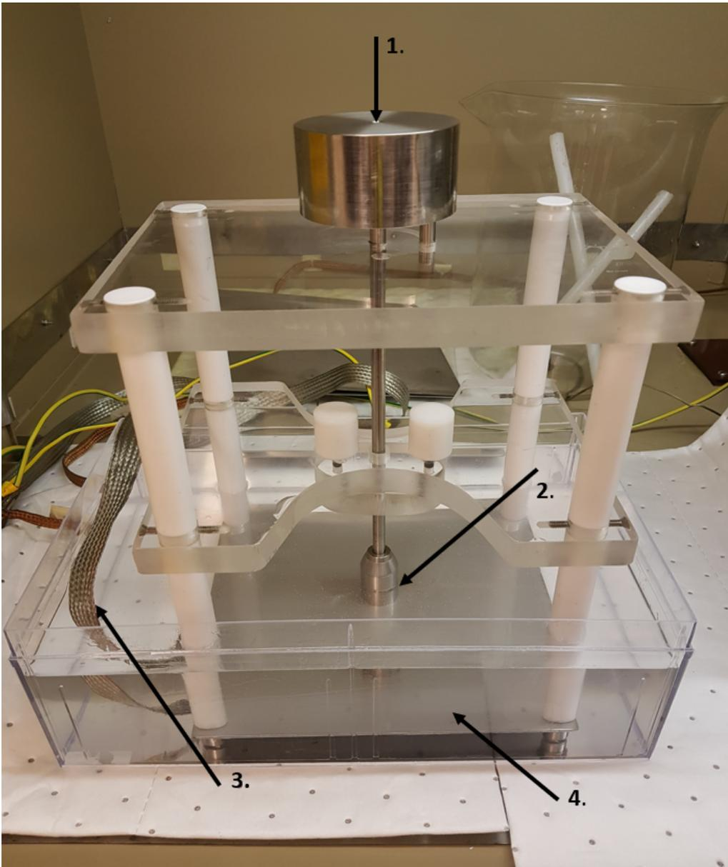
**Figure A.1:** High voltage test rig with standard electrodes, with explaining numbers - 1. Is where the voltage cable is connected. 2. Placement of material. 3. Grounding cable. 4. Silicone oil.
