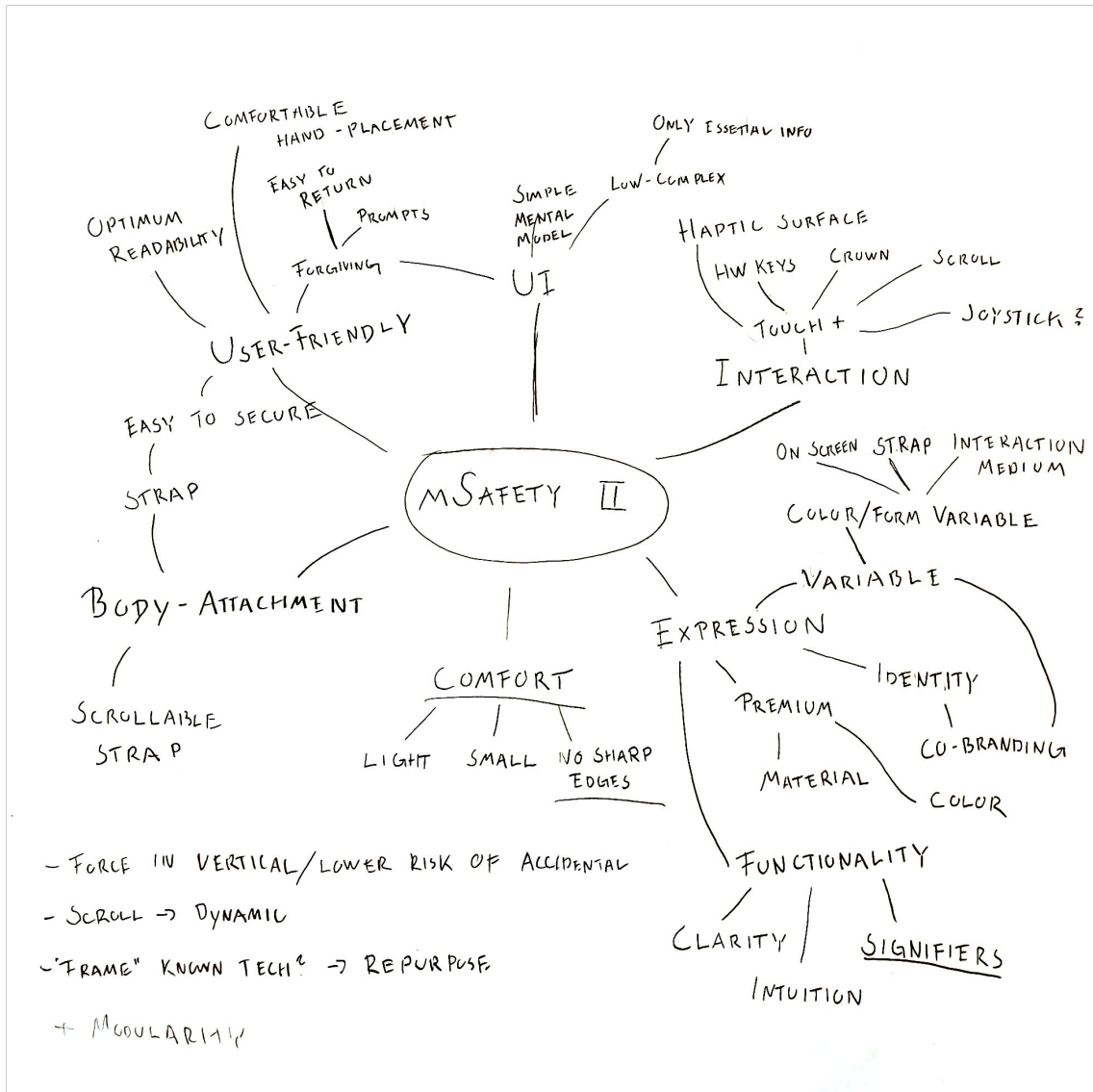
Figure 4.12: Mind map. It shows free thoughts and ideas of the different components of the product to be developed. Author's own illustration, 2021.
