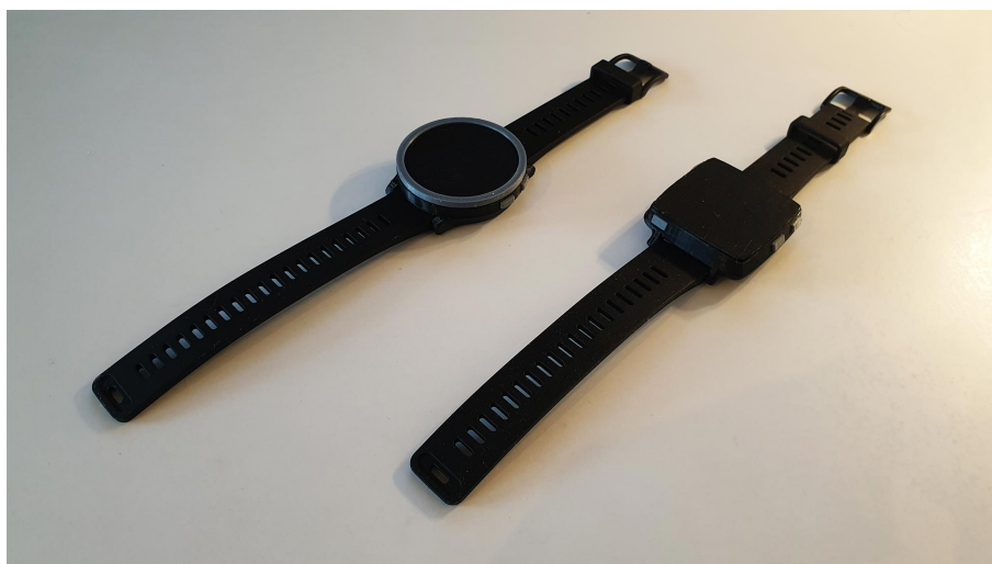
Figure 4.24: Two concepts printed and assembled with clickable buttons. Author's own illustration, 2021.
