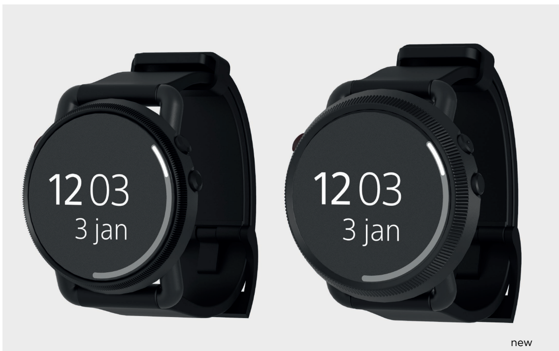
Figure 4.27: Final refinements. The new version is shown closest to the viewer and on the right. Major changes are in the rounded back, the angeling of the lugs, and their spacing from the buttons. Also, the surface area of the dial has been increased. Author's own illustration, 2021.
