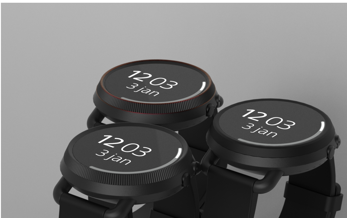
Figure 4.30: Various dials. The one closest to the viewer is designed for the industry. Behind it, with accent coloring, is the dial for leisure activities. The softer dial on the right is for the healthcare domain. Author's own illustration, 2021.
