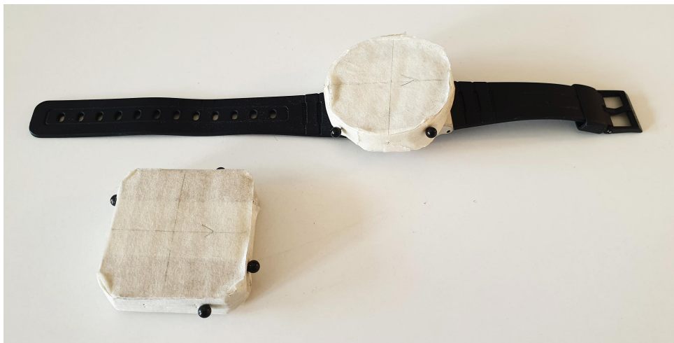
Figure 4.17: Cardboard mock-Ups. The black pins were used to test the reachability of different layouts. Author's own picture, 2021.
