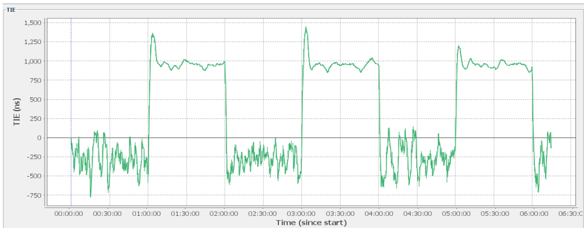
Figure 4.29: Proposed system performance for test case 2. As was expected from the observations made using the MTIE plots, the system's TIE performance is substantially improved. The proposed solution provides lower values for the TIE and better overshoot performance.
