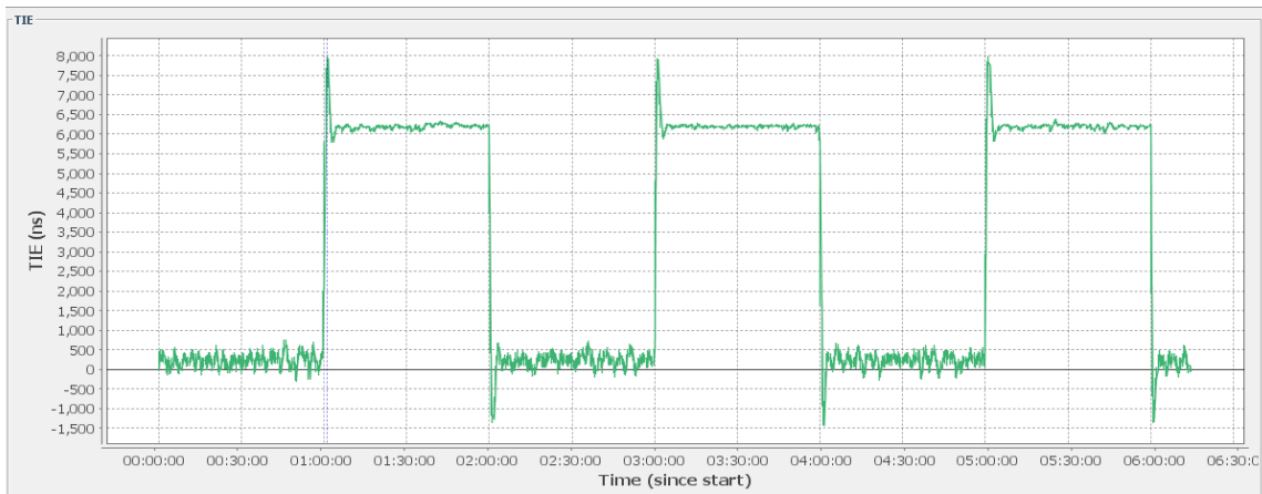
Figure 4.28: Reference system performance for test case 2. The timing error in this second test case is almost 8 times higher than the one observed in test case 1. This test case is also indicative of the overshoot performance of the reference system which is quite poor.
